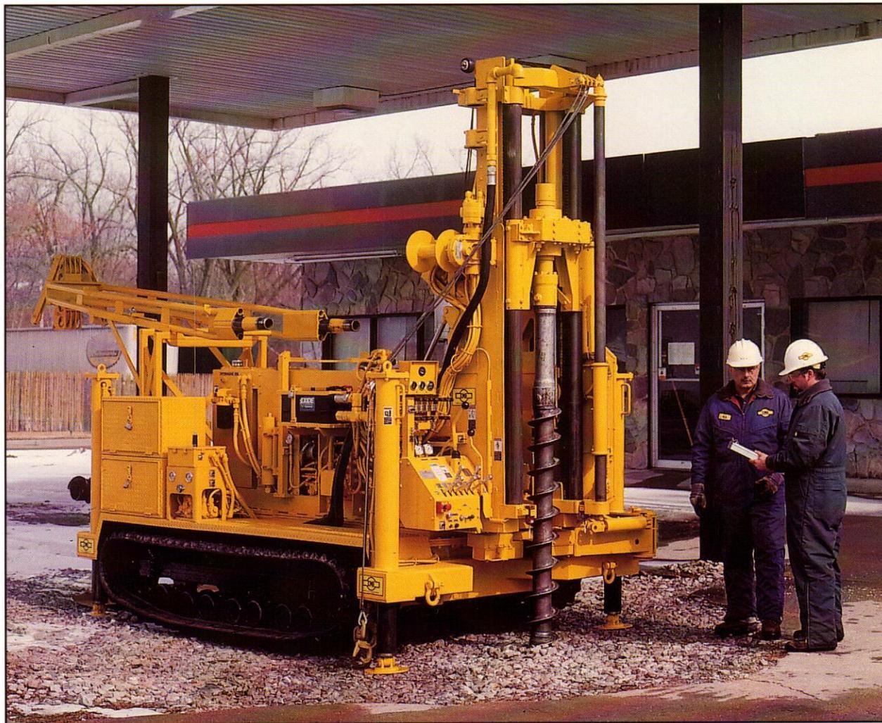
The CME-55LC has a unique feed and retract system and a quick disconnect mast that allows you to work under service station canopies, bridges or other overhead restrictions. The overall set-up height with the mast disconnected is only 12 foot, 1 inch when mounted on the CME-300 tracked carrier. A truck mounted CME-55LC is also available.
